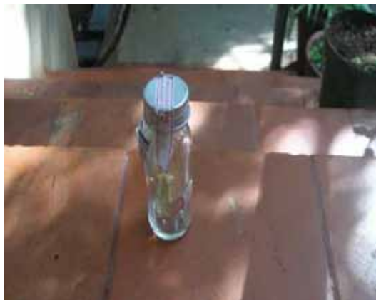
H 2 S strip test bottle: If the water turns black in the bottle then it is micro-biologically contaminated.
