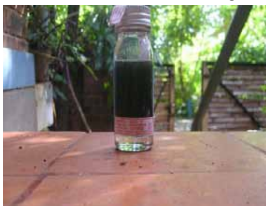
H 2 S strip test bottle: If the water turns black in the bottle then it is micro-biologically contaminated.
